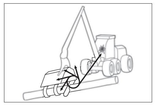
Chain shot can cause chain parts to be thrown in many directions, especially those along the plane of the saw bar.
