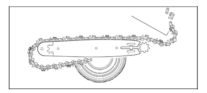
3. At the peak of the whip, chain parts may break loose and be ejected at high speed, especially if the free end of the chain strikes the saw box.
