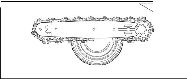
1. After a chain break, the "free" end of the chain begins to whip away from the break.
