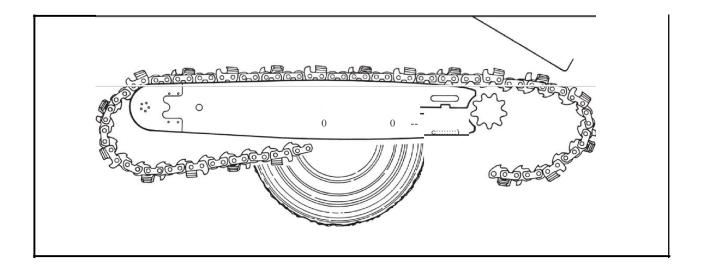
2. If the chain is not contained by the saw box or an energy-absorbing guard, the broken chain's free end can speed up rapidly and carry immense dynamic energy.
