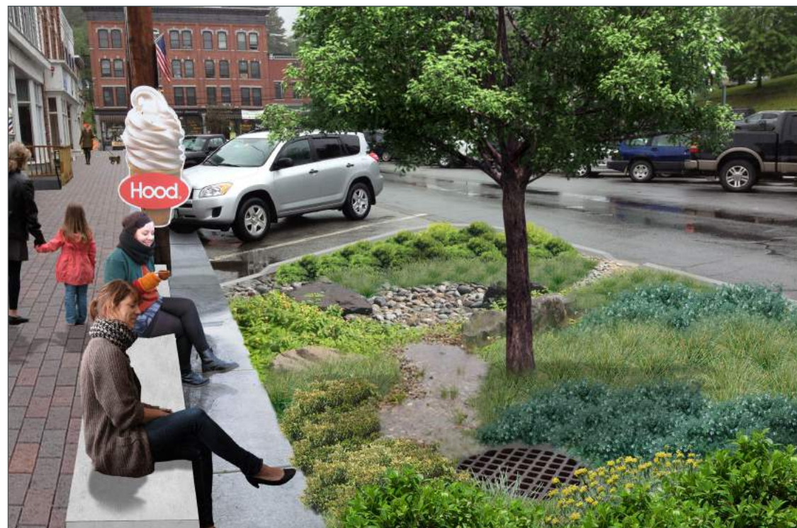
▲ RETROFIT OPPORTUNITY: The same downtown main street retrofitted with stormwater curb extension. In this example, the stormwater curb extension also uses space that is already striped as “no parking”.
