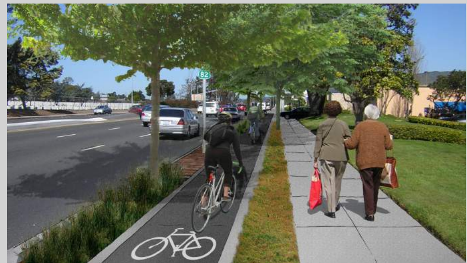
▲ This bold Green Street project separates bike, pedestrian, and vehicular movements with vegetated swales and stormwater planters.
