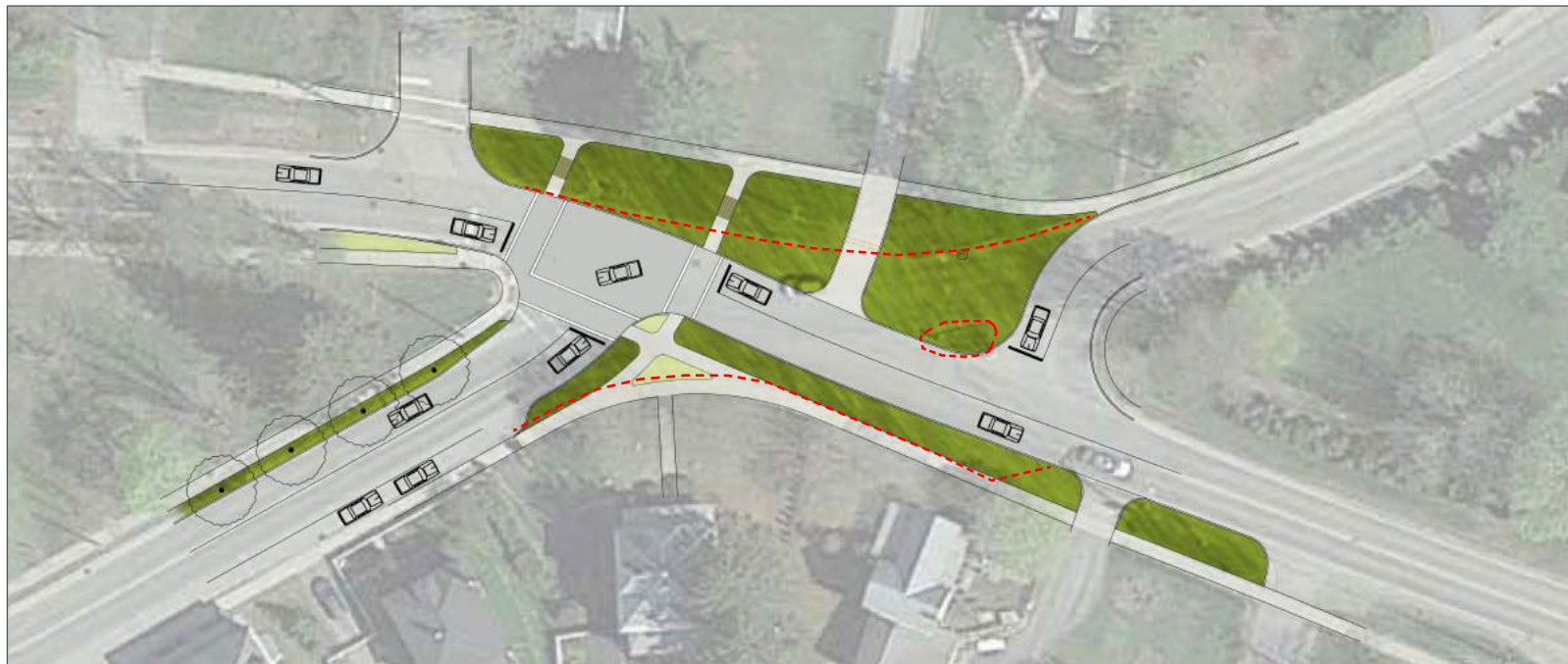
▲ RETROFIT OPPORTUNITY: The same residential streets in Middlebury retrofitted with multiple rain gardens once the intersection is realigned.
